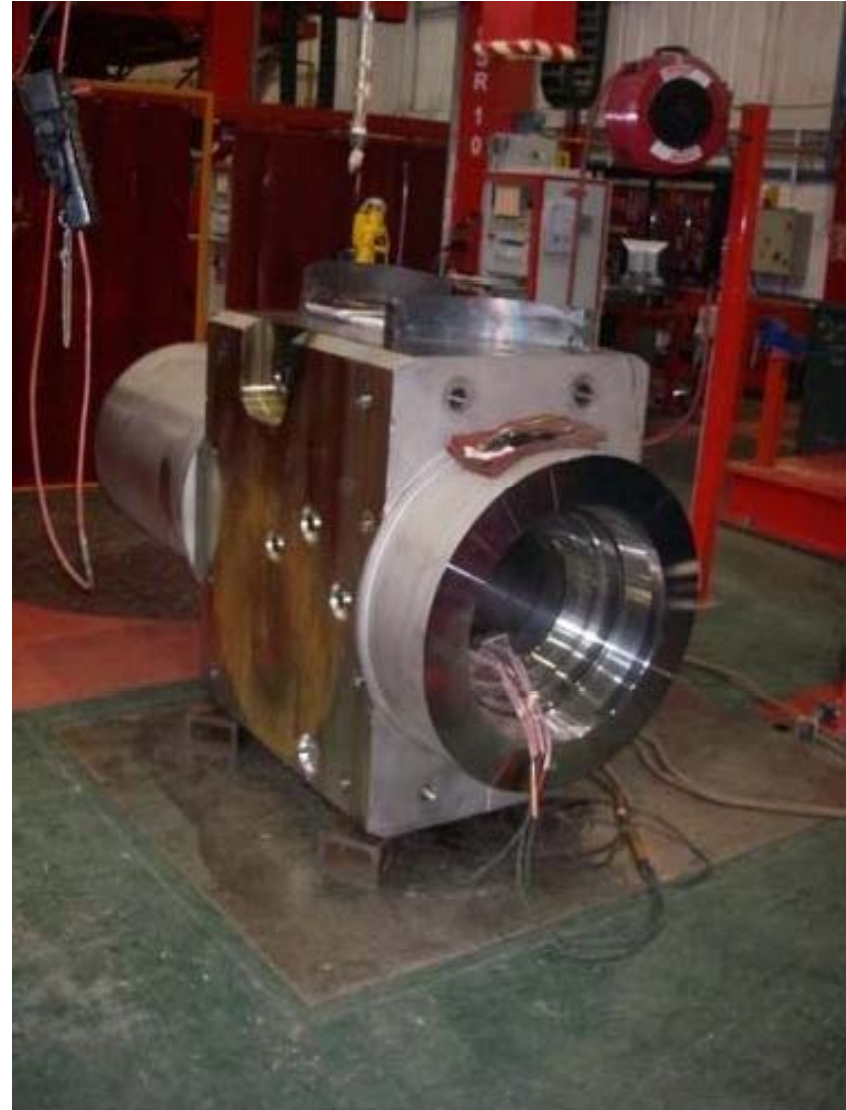
Valve for the Jette subsea system
