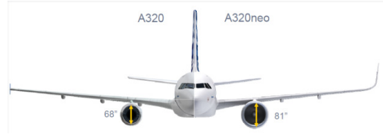
The primary visual differences between the A320 and the NEO are larger engines and new wingtips called “sharklets”
