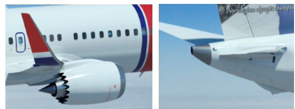
Noise reducing «chevrons» at the trailing edge of the engines and a more aerodynamic tail design are the most distinct visual changes.
