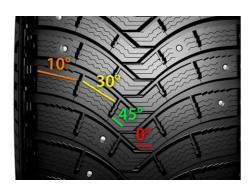
Sipes are laid out at angles that vary from 0° to 45°. This ensures progressive grip in all situations, whether cornering or driving straight ahead, for better handling and easier steering.
