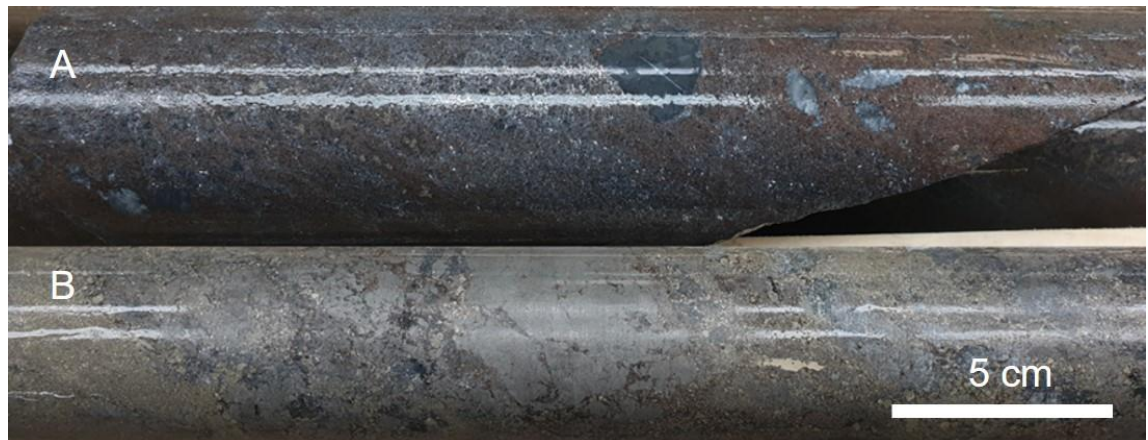
Figure 3. Core photos showing the mineralization from discovery holes STROM12. A: Massive sulphide mineralization dominated by a mineral assemblage of sphalerite, pyrrhotite, galena and sulphosalts at 310m. B: Massive arsenopyrite and pyrite mineralization with minor amounts of sphalerite, galena, sulphosalts and chalcopyrite at 350m.
