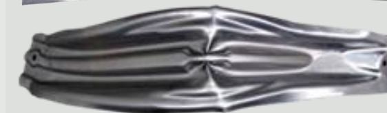
Prototype Door-beam Docol CR 1700M-EG
