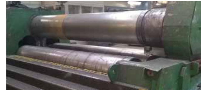
PLATE ROLL BENDING Max width 4,500 mm. Max thickness 110 mm.
