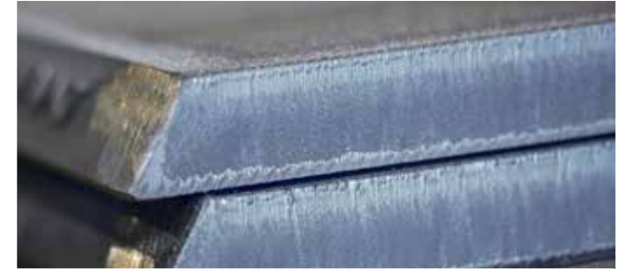
BEVELLING Max thickness 140 mm. Max length of bevel 12,000 mm.
