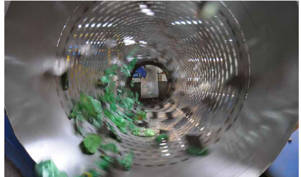
Machinery separating caps and rings from bottles (Polygenta Trommel)
