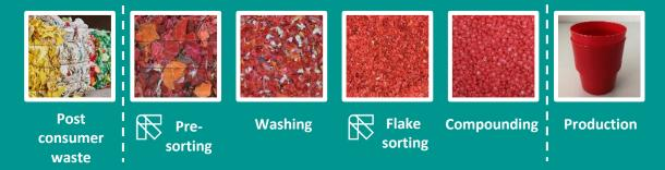
The demo plant covers the process from post consumer waste to production of recycled polymers.
