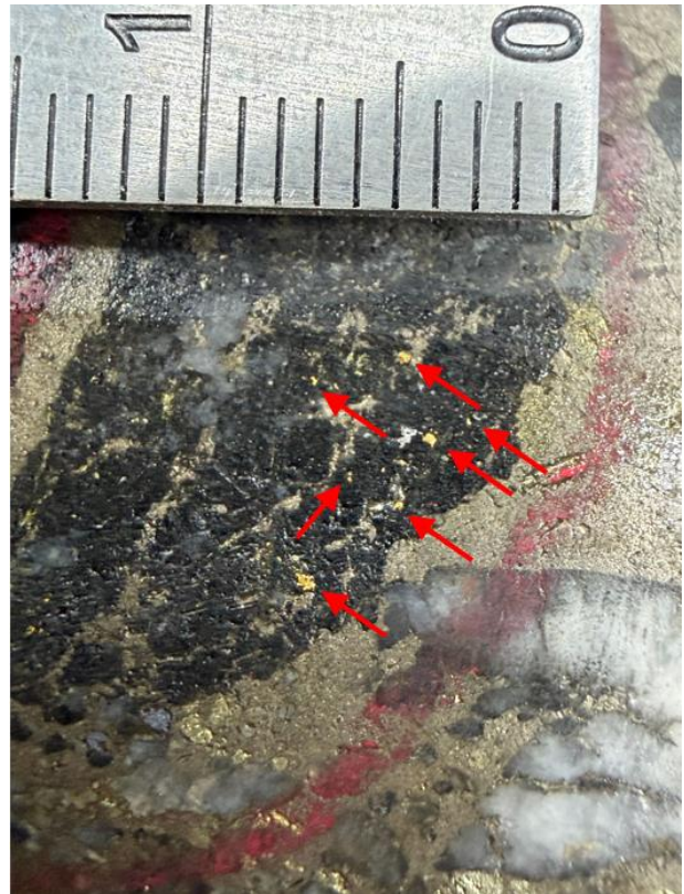
Figure 2: Drillhole photograph taken of drillhole PAL0406 from the Palokas Au-Co zone of mineralization from Rajapalot, where visible gold is observed at 111m downhole depth. Gold grains have formed alongside the salvages of a pyrrhotite-quartz vein.
