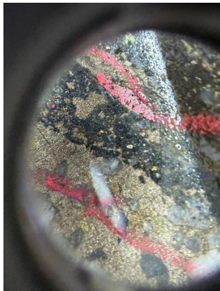
Figure 2: Drillhole photograph taken of drillhole PAL0406 from the Palokas Au-Co zone of mineralization from Rajapalot, where visible gold is observed at 111m downhole depth. Gold grains have formed alongside the salvages of a pyrrhotite-quartz vein.
