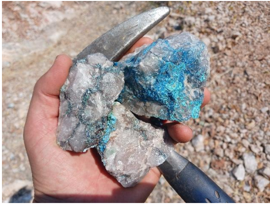
Cu mineralisation hosted in quartz veins
