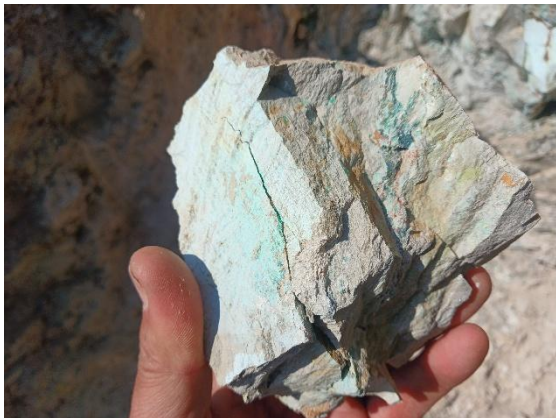
Disseminated Cu-mineralisation in reduced siltstone
