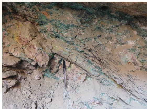
Exposed supergene Cu-mineralised horizon by artisanal workings.
