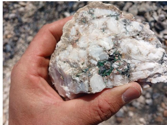
Hypogene and Supergene Cu mineralisation hosted in calcite veins
