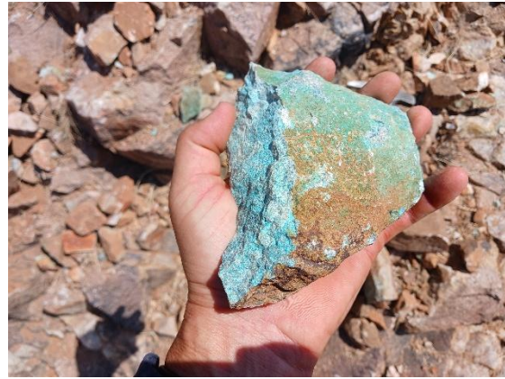
Disseminated Cu-mineralisation in quartzite from the Nosib Group
