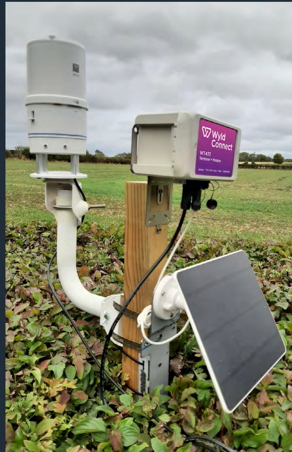
Image: Wyld Networks' innovative Satellite Terminal with integrated weather station, launched earlier this year.
