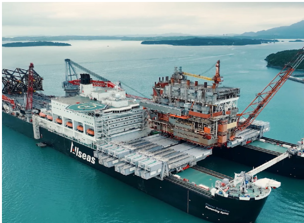
Aker BP’s Valhall platform on its way to our Stord, Norway facility to begin the decommissioning and recycling process.
