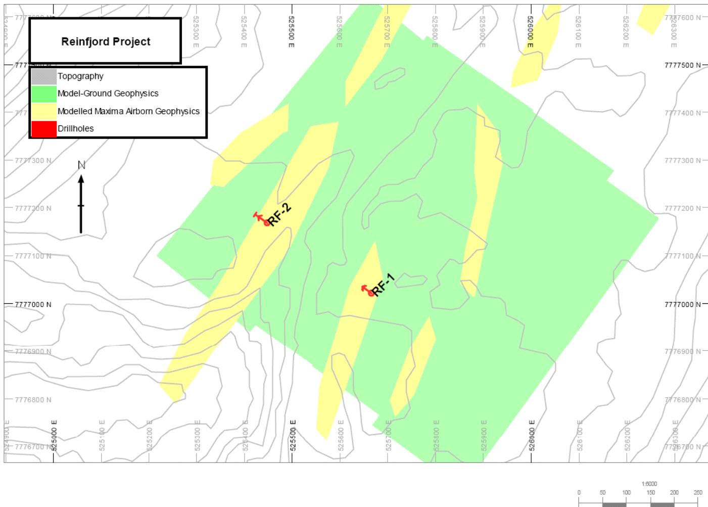
The figure presents the modelled conductive plate from ground geophysical survey (green) and modelled peak conductivity from the airborne geophysical survey. Red arrows show the positions of the drill holes.
