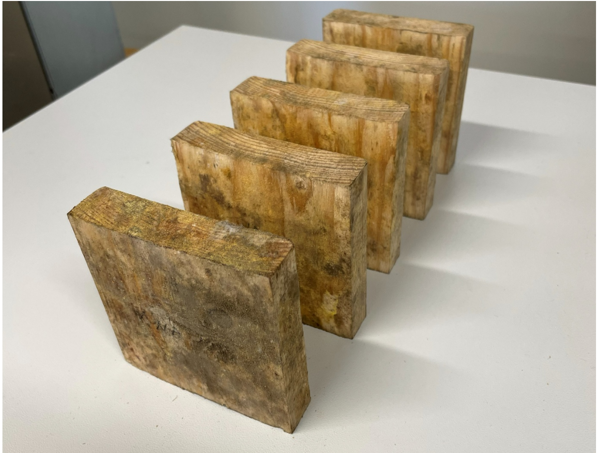
Figure 18: Severe mould growth on 100 mm samples after conditioning of NN-wood.
