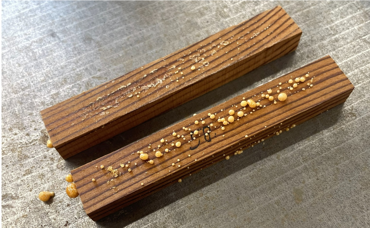
Figure 19: Yellow droplets formed on surface of Woodsafe WFX samples during drying at 103 °C.
