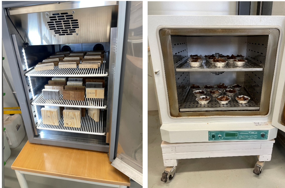
Figure 7: Cabinets used for conditioning of the specimens and oven drying of specimens.
