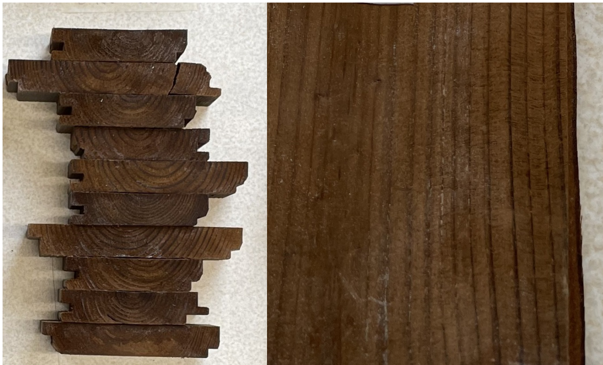
Figure 17: Salt crystals formed during conditioning on end surfaces and interior surfaces of samples protected from precipitation treated with Burnblock (Material C).
