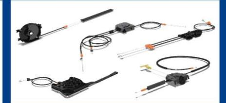
Cabling systems for all aspects of the vehicle where movement or release is a function of the system
