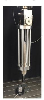
The Cuttings Transport module was developed in 2016 and the chain based transporting system passed relevant endurance testing. It also proved to handle dry and wet cuttings in a satisfactory way.
