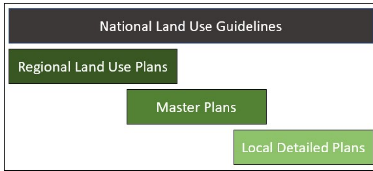
Figure 20-6. Land Use Plan Hierarchy as defined in Land Use and Building Act (132/1999) and Decree (895/1999).
