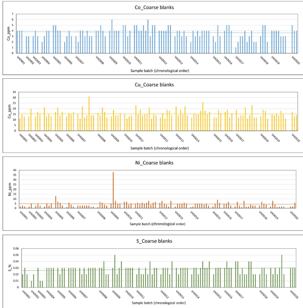
Figure 8-4 Coarse blank analysis results of the 2020 FinnCobalt drilling campaign, sorted by submitted sample batch in chronological order.
