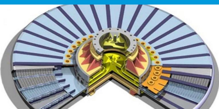
The ESS tungsten target wheel is a novel design. It will measure 2.5 meters in diameter and weigh 4 tonnes.
