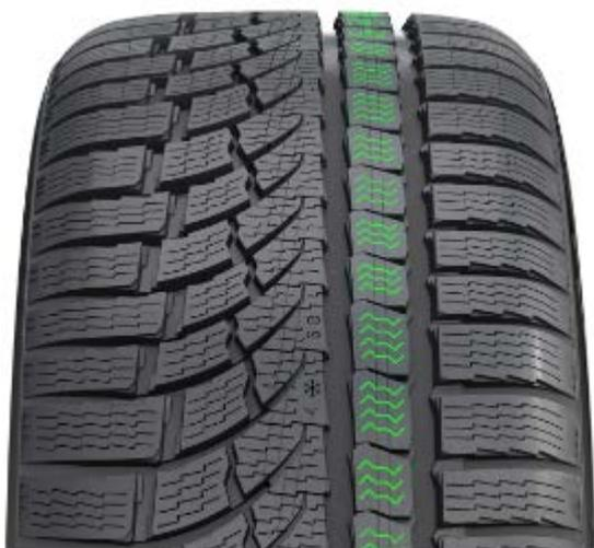
The centre area is dominated by a sturdy longitudinal rib consisting of tread blocks with jagged sipes that resemble the footprints of a centipede. The staggered 3-dimensional **Centipede Siping** offers maximum contact surface and works with full effect at different turning angles, increasing grip on snow and slush and improving control.
