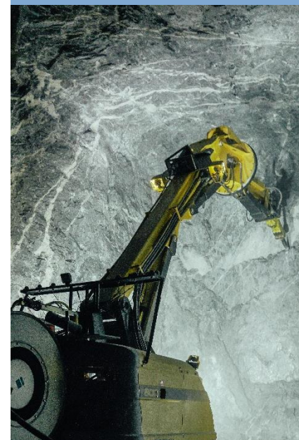
Remote-controlled scaler in Kankberg
