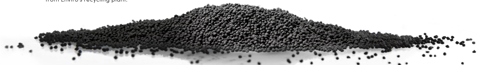
Recovered pelletized carbon black from Enviro's recycling plant.
