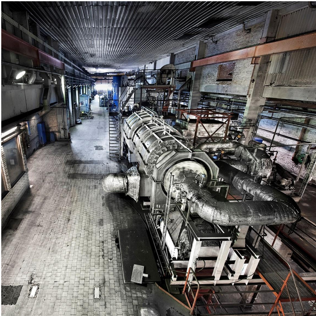
This shows a picture of our plant in Åsensbruk. Up close the pelletizing and drying section of our recovered carbon black is to be found.
