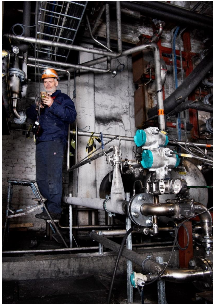
Process engineer Carl-Johan Pihlgren is performing calibration of a valve for the handling of oil in the plant at Åsensbruk.
