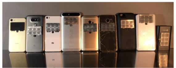
myFC's integrated fuel cell, here in the iPhone 7, LG G5, Xiaomi Mi5, Huawei Nexus 6P, HTC 10, Samsung Galaxy S7, Mophie Juice Pack, GP Powerbank, and Anker PowerCore+.
