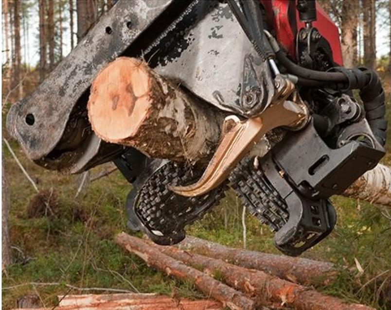
"The TP-Roller design is a complete departure from other feeding rollers," said Timo Penttimies, developer of the TP-Roller. "The rollers are laser-cut discs made of high-strength steel, with relief holes and integrated sprocket teeth. They range from four to 11 discs per roller, depending on the width and use, and also have space for a cleaning device.
