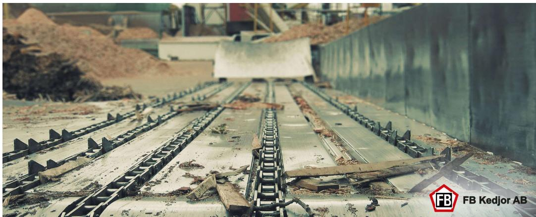
Using Hardox® HiAce as a liner in chain conveyors working in acidic environments gives substantially longer service life.
