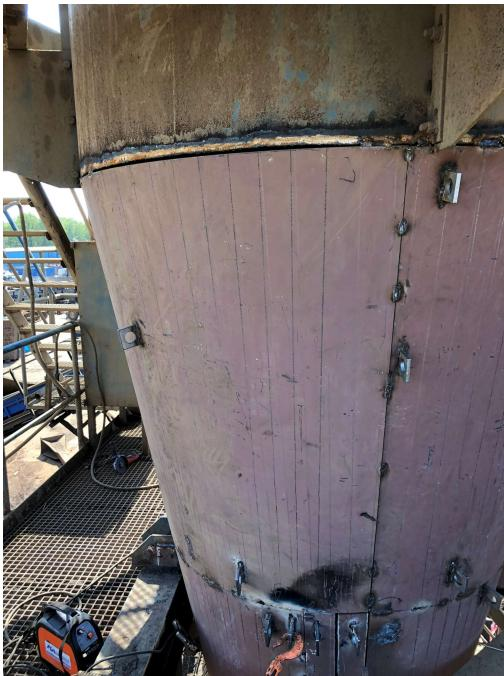
Hardox® HiAce replaced the earlier solution with structure plate and wear plate made of S355 (A36) in cyclones at a Stena Recycling plant.
