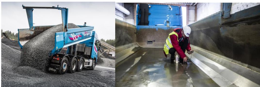
*The dump body in the pictures is made with Hardox® 500 Tuf in the bottom plate. It has transported over 88 million pounds (40,000 metric tons) of crushed rock during more than a year with very low wear. Measuring the thickness at the end section of the 0.236 in. (6 mm) bottom plate showed an average wear of only 5%.*
