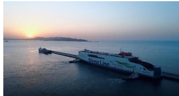
In total, Stena Line will be operating five E-Flexer vessels, with two of them being the extended version. The fourth in the order has now been delivered. Compared to the basic design, the ferry has been extended by 36 meters. With the extension, the ferry is 240 meters long and has an increased capacity of 50% more cabins, 30% more passengers and 15% more cargo. Loading and unloading are streamlined with a drive-through configuration for both car decks.
