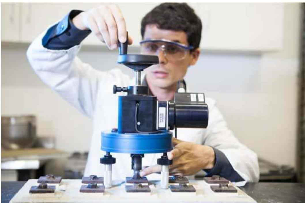
Practical test at Wacker Química do Brasil's technical center: In the newly expanded lab for dispersible polymer powders, an employee is testing the tensile bond strength of tile adhesives, which is significantly increased by WACKER's dispersible powders. In close collaboration with customers and partners, the technical center is developing and testing new products and formulations for the South American market (photo: Wacker Chemie AG).
