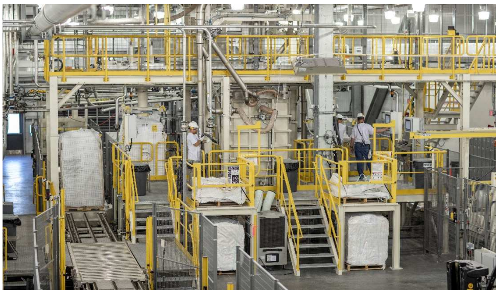
The filling system for pyrogenic silica at the Charleston site. A fully automated process is used here for packaging pyrogenic silica in so called Big Bags. (Photo: WACKER)
