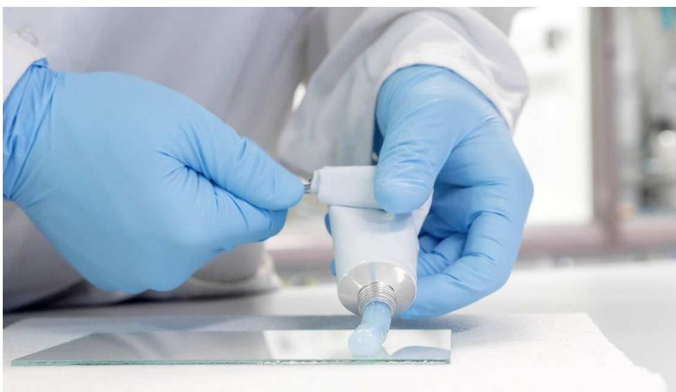
Industrial adhesives formulated with WACKER's HDK® H21 pyrogenic silica are extremely resistant to sagging and do not run on sloping or curved bonding surfaces. (Photo: WACKER)
