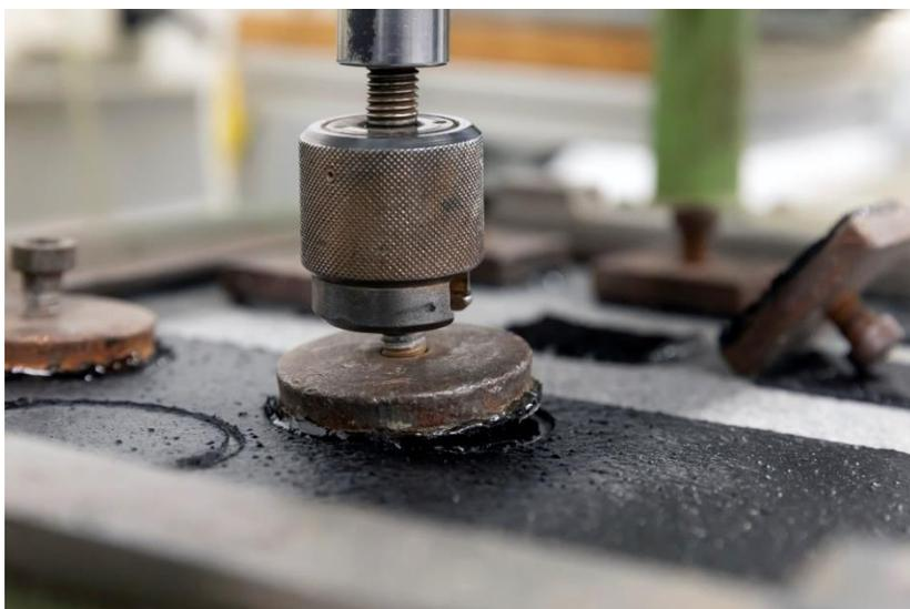
Tensile adhesion strength test: polymer modification meant that the tensile adhesion strength rose by as much as 60 percent compared to conventional bitumen emulsions. (Photo: Wacker Chemie AG)
