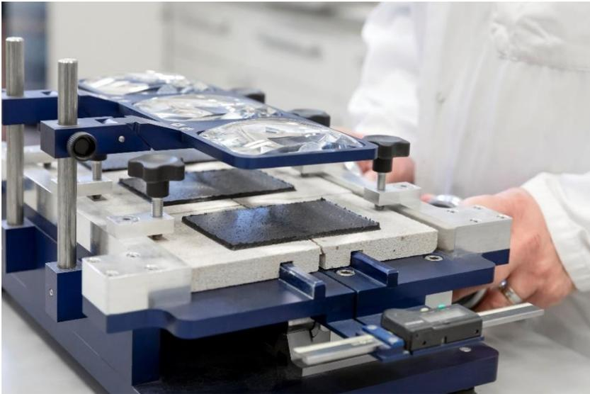
Examining crack-bridging: when exposed to stress, the polymer-modified bitumen emulsion has to endure cracks in the concrete substrate. (Photo: Wacker Chemie AG)
