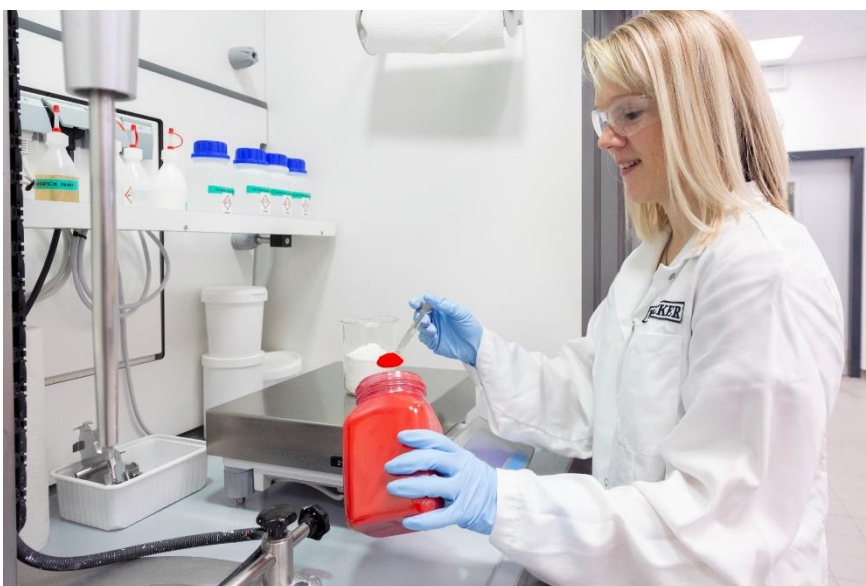
A WACKER lab assistant adds pigments to a dispersible polymer powder. (Photo: Wacker Chemie AG)
