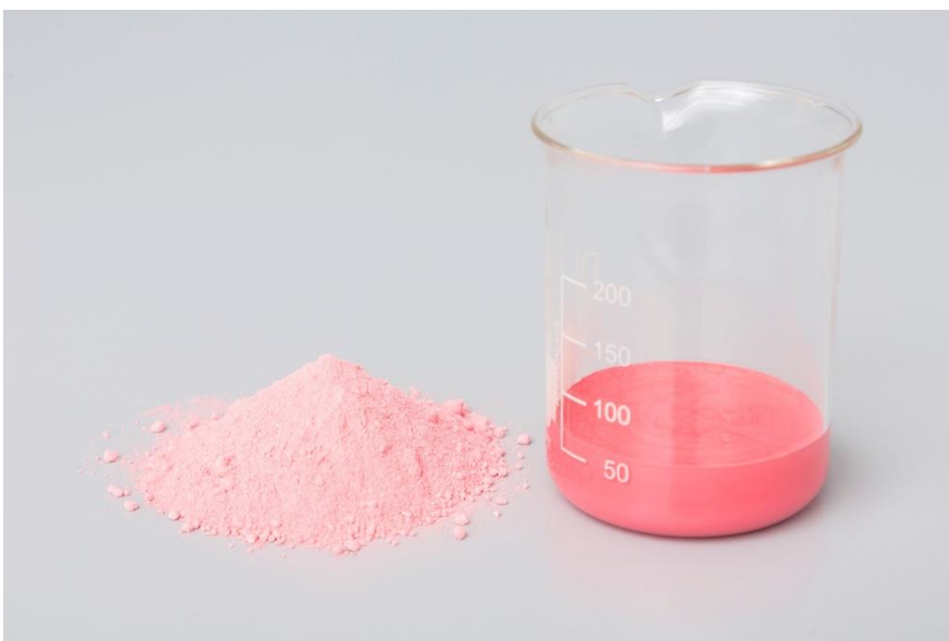
Paint containing NEXIVA® in powder form (left) and redispersed with water (right). (Photo: Wacker Chemie AG)
