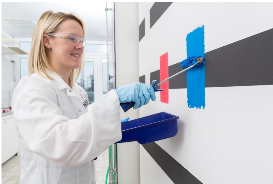
A WACKER lab assistant checks the hiding power of paint.
