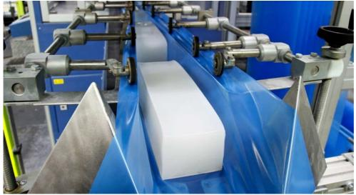
WACKER, the Munich-based chemical group, is showcasing two new hardnesses for its ELASTOSIL® R *plus* 4001 high consistency silicone rubber line at the 2018 German Rubber Conference DKT in Nuremberg. Providing a Shore A hardness of 20 or 90, respectively, these grades exhibit outstanding elasticity properties. (Photo: WACKER)
