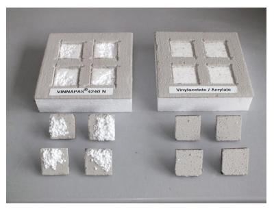
Laboratory experiments show that the new dispersible polymer powder VINNAPAS® 4240 N has a better tensile adhesive strength and stripping resistance than conventional market products after just one day. This ensures a very strong adhesive bond between an EPS panel and masonry in external thermal insulation composite systems. (Source: Wacker Chemie AG)
