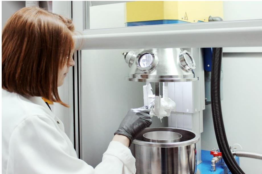
Highly specific tests can be performed in the new laboratory in Moscow. The image shows lab assistant Ekaterina Aleksandrova using a planetary mixer to produce a low-modulus sealant with silane-modified polyether as a binder. (Source: Wacker Chemie AG)
