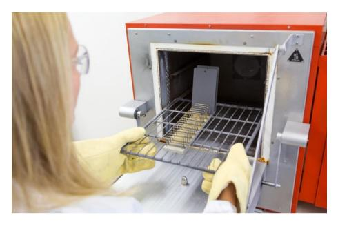
The thermal resistance of the new SILRES® REN70-M binder is tested in the WACKER lab by coating steel plates with a paint containing the binder and heating them up to 650 °C (photo: Wacker Chemie AG).
