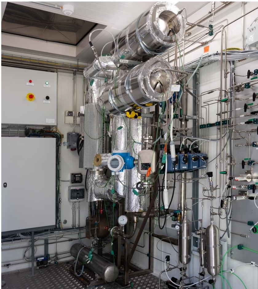
Picture 2. VTT's pilot equipment for converting carbon dioxide into synthesis gas. Synthesis gas produces ethylene and propane gases for polymer production.
