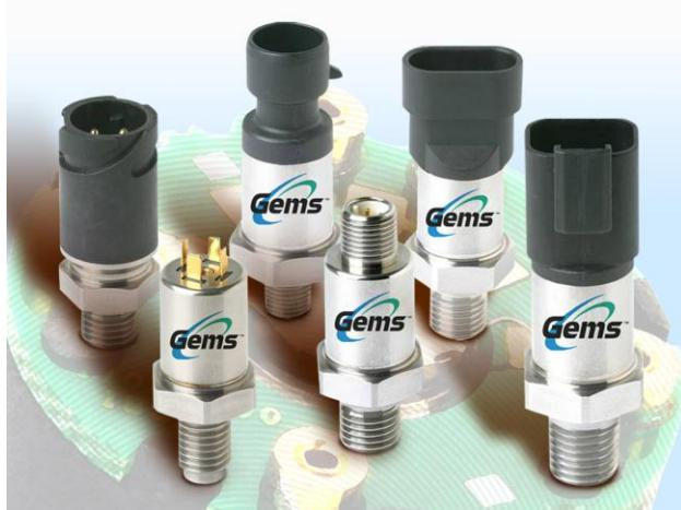
Built using 17-4PH stainless steel wetted parts, the 31CS and 32CS series also features proven Sputtered Thin Film sensing technology, and ASIC-controlled thermal compensation and signal conditioning. The 31CS and 32CS are identical in their compact and durable design, with the exception of a thicker diaphragm and a pressure restrictor on the 32CS series. This enables the
