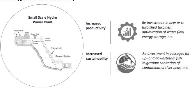
Figure 29 Schematic picture of small scale HPP and examples of measurers to restore ecological qualities and technical upgrades for increased productivity
