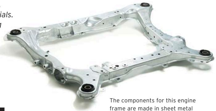
The components for this engine frame are made in sheet metal presses and then assembled in welding cells and machined before being delivered to a car maker.
