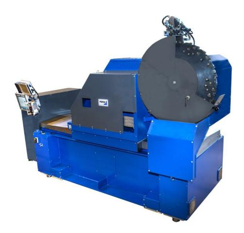
**PEMA CM 55** is an advanced milling machine for joint preparation of circumferential seams. The new innovation increases welding quality and efficiency significantly, while it provides easy milling process. Additionally, the features included in PEMA CM 55 are specifically designed to reduce defect rate.
