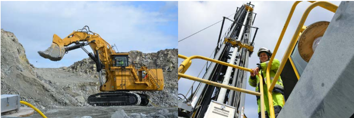
The Cat hydraulic shovel, model 6060, and the drill rig from Atlas Copco in operation.
