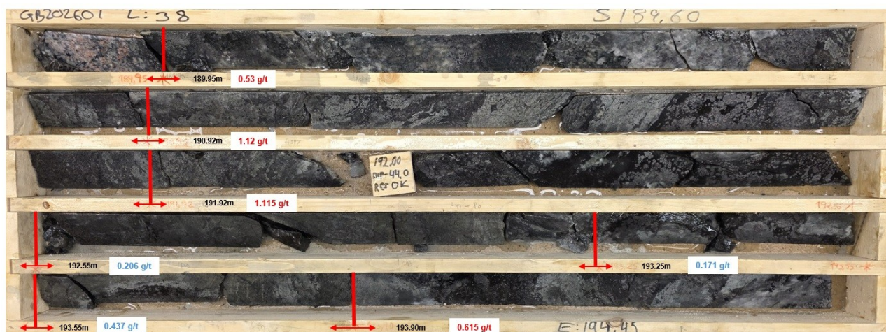
Image 1. Drill core from GB202601, box 38, 189.95 to 194.45 metres. This is where the gold zone begins.
