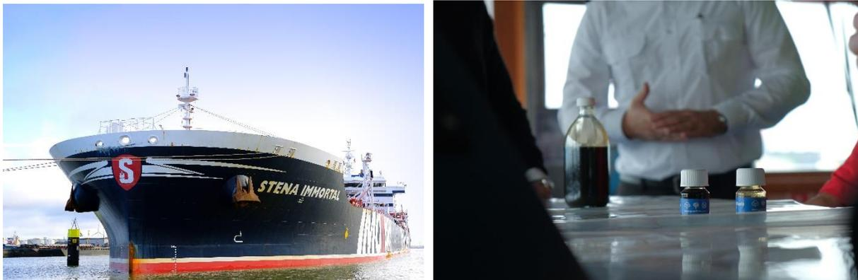
The trial was completed on the *Stena Immortal* as she ran in typical commercial operation. During the trial, BFO was tested in tanks, storage and as it was burned in the engines, the fuel was again proven to be a technically compliant alternative to the fossil default for oceangoing tanker vessels.
