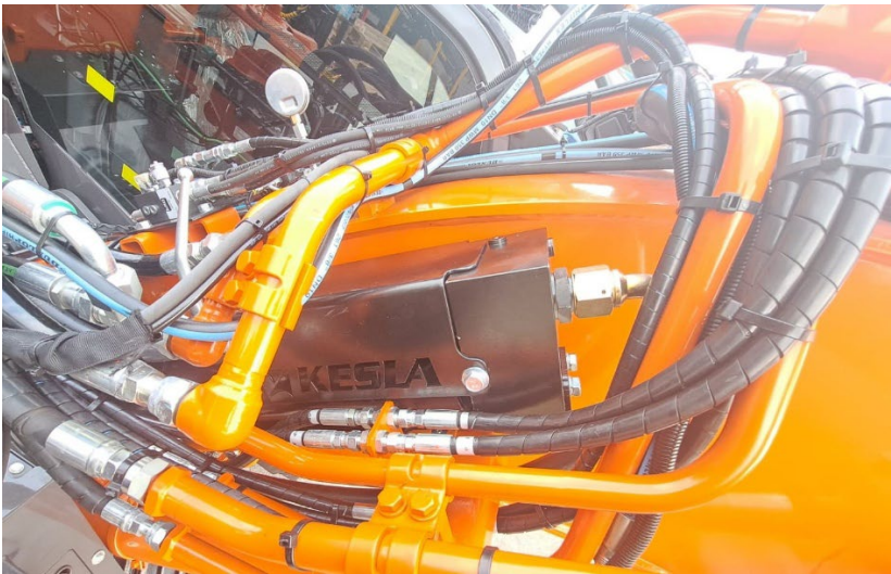
Picture 1. KESLA powerB pressure accumulator system
