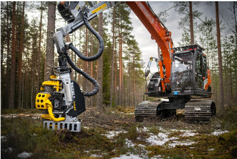
Picture 1. KESLA 19RH-III harvester head & Hitachi excavator
