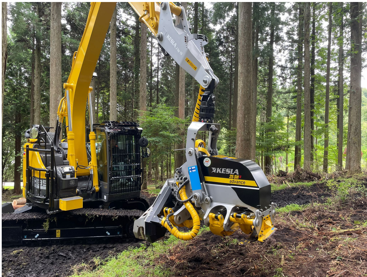
1. Sumitomo SH135 & KESLA 25SH-II Advance harvester head, Japan.
