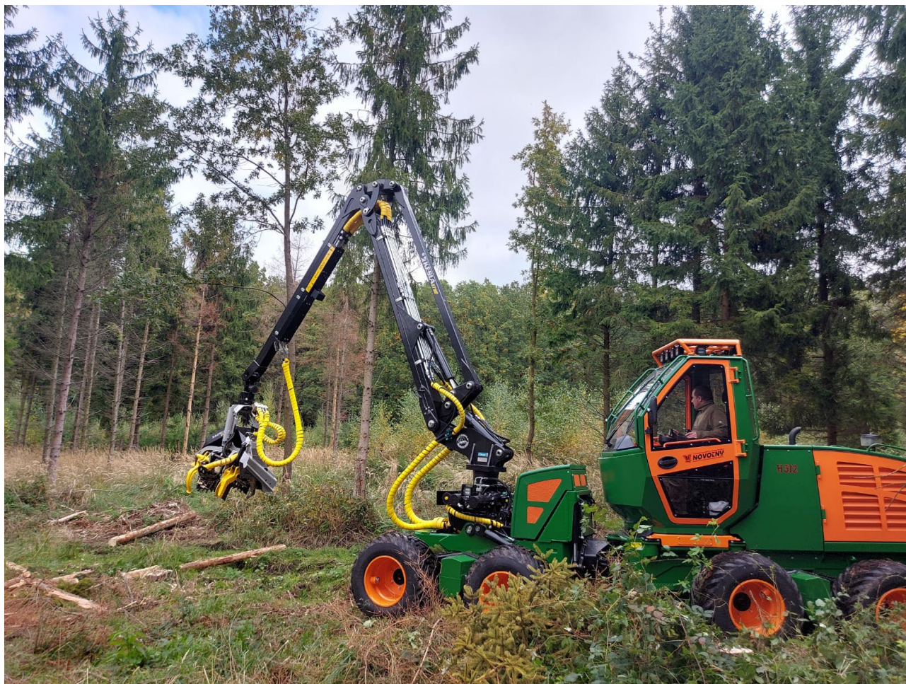
1. Novotny 8WD & KESLA 16RH harvester head and KESLA 671HF harvester crane. Customer - Jacub Strojnan, CZ.
